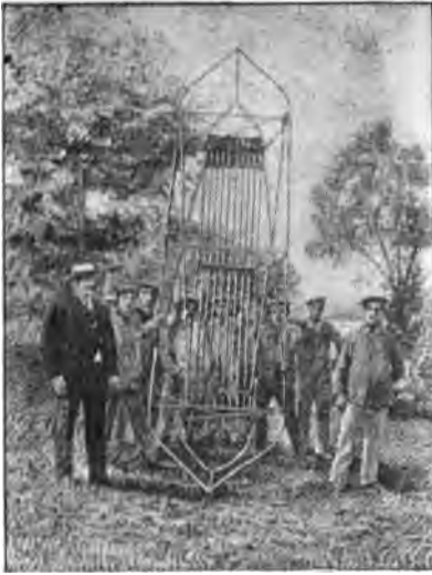
NEW PORTABLE BOAT MADE OF CAVALRY LANCES FOR USE IN GERMAN ARMY.
